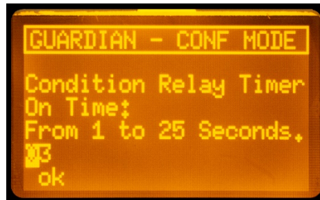
Figure 25: Condition Relay dwell time
